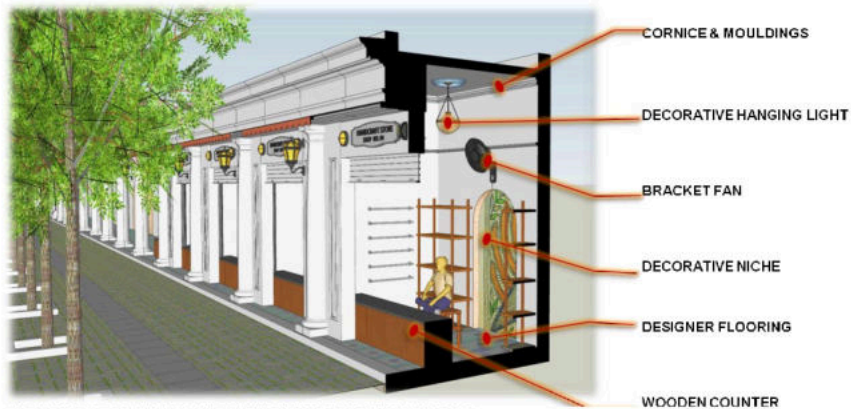
FIGURE 37 SECTIONAL VIEW SHOWING SHOP INTERIORS
