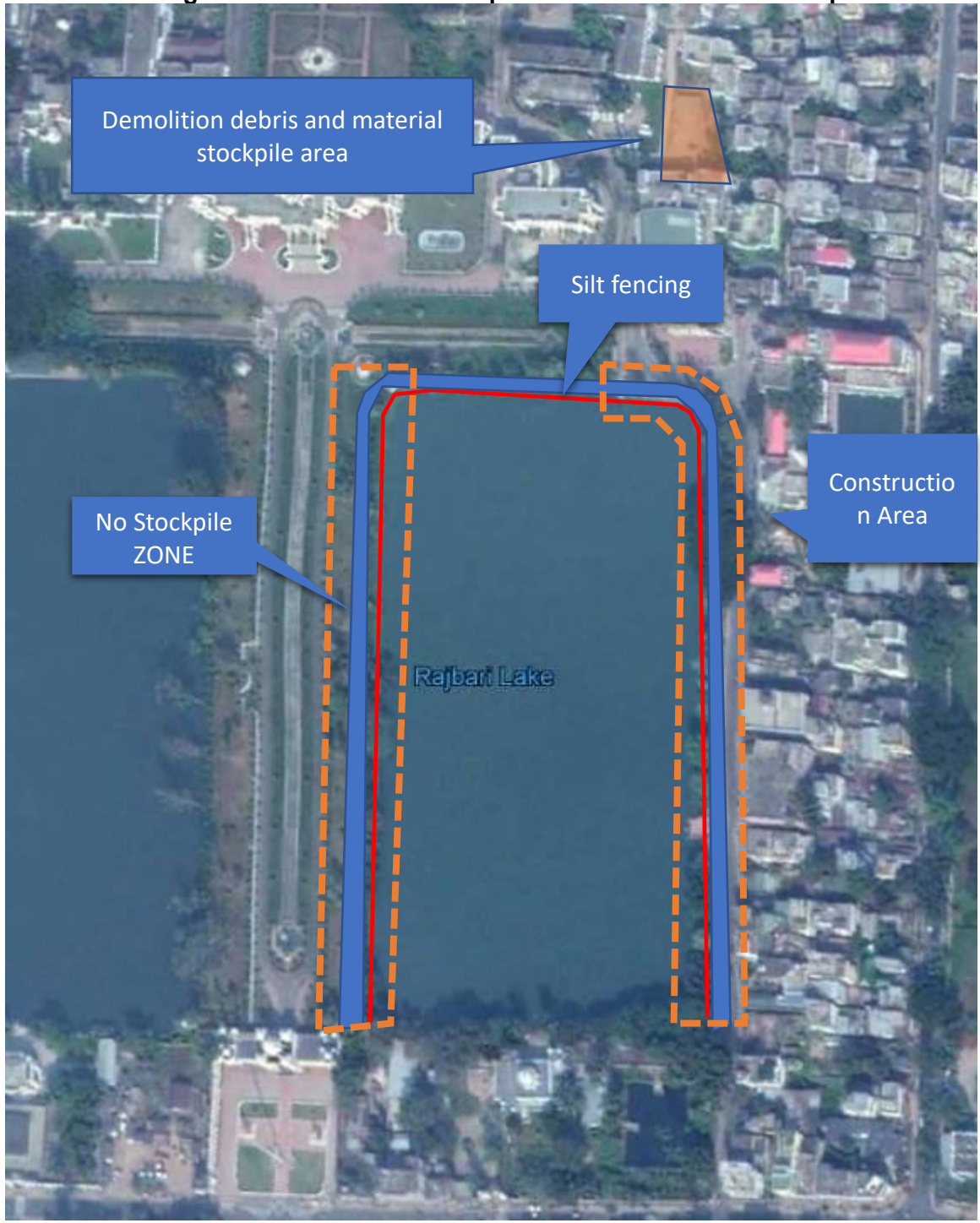
Figure 32 Construction site plan for Eastern Lake Development
