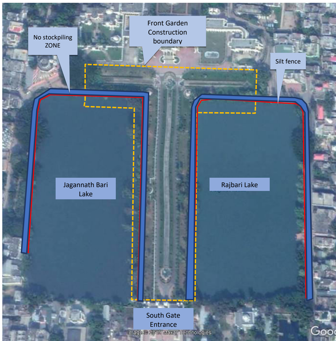
Figure 28: Construction site plan for Front Garden
